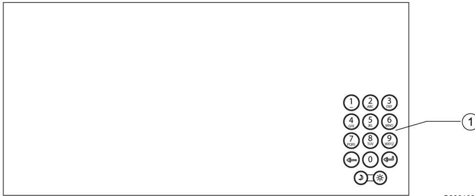
Figure 6. The keypad on the control panel.
